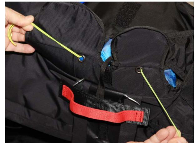
Push the metal pins on the deployment handle into the elastic loops. After this operation, the thin cord must be removed. This is very important. Remove the cord slowly and carefully in order not to damage the elastic loops by creating excessive friction. After completing this, the handle should be inserted below the elastic cover. Position the final cover flap so that it fits closely and covers the Velcro on the deployment handle.
